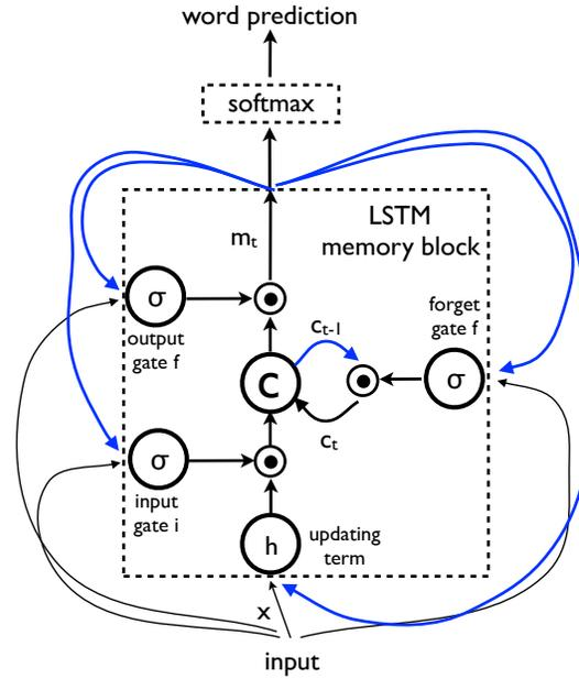
Figure 2. LSTM: the memory block contains a cell  $c$  which is controlled by three gates. In blue we show the recurrent connections – the output  $m$  at time  $t - 1$  is fed back to the memory at time  $t$  via the three gates; the cell value is fed back via the forget gate; the predicted word at time  $t - 1$  is fed back in addition to the memory output  $m$  at time  $t$  into the Softmax for word prediction.
