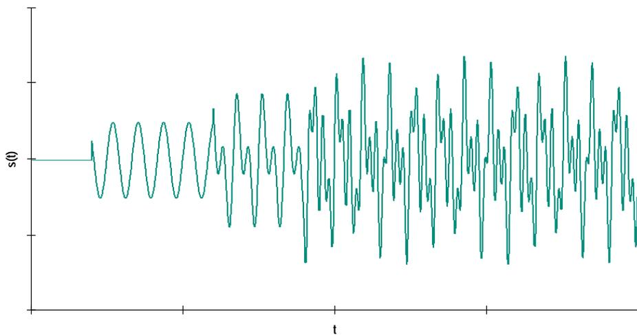
**Fig. 19.** Three sinusoids with different starting times.
