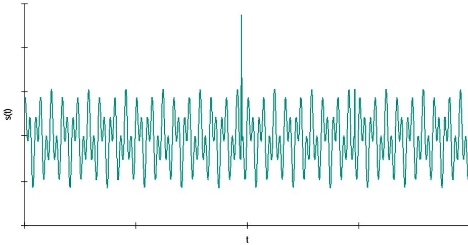
**Fig. 16.** Two delta functions and two sinusoids.
